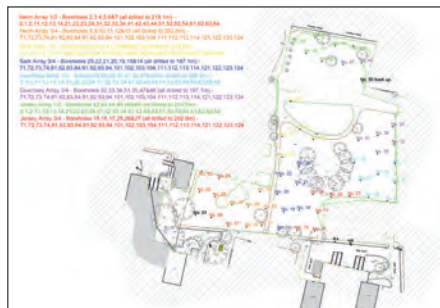
As installed drawing showing the location of the boreholes drilled for four of the tower blocks at the Channel Islands and Kettering Road project.
